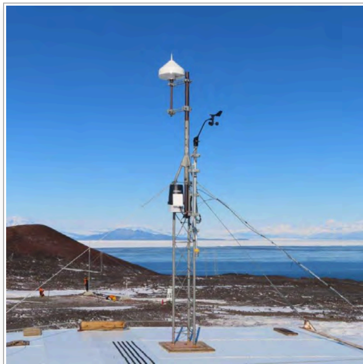
Multi-GNSS data collection system to capture space weather activities. Photo courtesy of University of Colorado Boulder.
